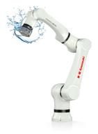
**Well Protected:** Thanks to its compact and robust design, integrated cables and IP66 rating, the CL Series can be used in all kinds of harsh environments that may not be suitable for other collaborative robots.
